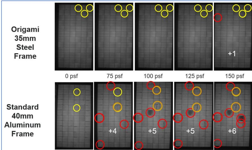
Figure 8 – 1/5<sup>th</sup> Strut-Rail Downforce EL Test Results
