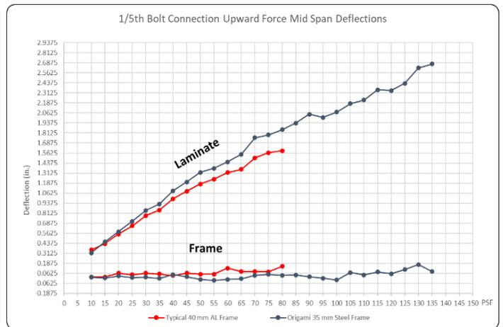
Figure 6 – 1/5<sup>th</sup> Strut-Rail Upforce Deflection Results
