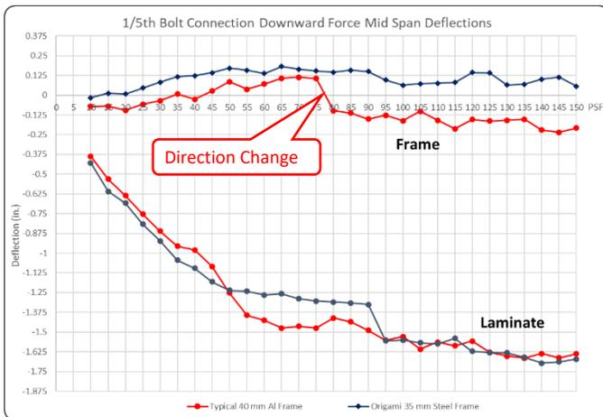
Figure 5 – 1/5<sup>th</sup> Strut-Rail Downforce Deflection Results
